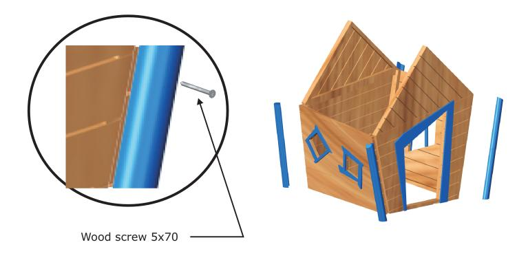
**Step 10: Place the assembled house on the platform. Corner decorations need to fix with the short post below floor.**
