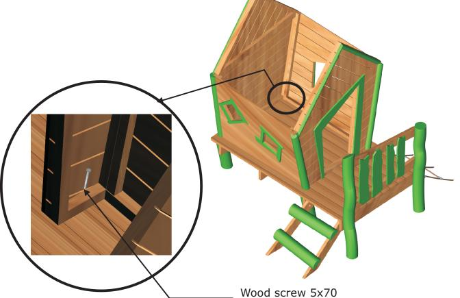
Step 12: Screw the chimney to one part of the roof, in the middle, aprox. on the third board counting from top.
