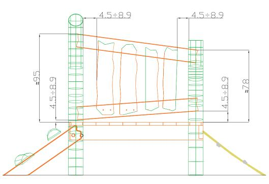
LARS LAJ<sup>®</sup> 13154 (12)Installation manual Step 15: Install roof. 1 - Wood screw 5x70 Wood screw 5x100
