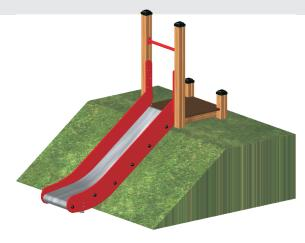
The hill must reflect the shape of the slide. The slide must be parallel to the hill: it must either lay flat on the slope or it can be elevated above the ground, but the space between should be 30-40mm. The space between the slide and the hill must be the same through its full length. It can not be narrowed downhill.
